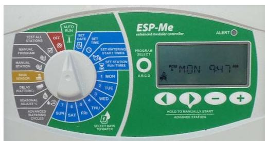
Irrigation Control is color coded; "Off" position is the red station, just to the left of center.
